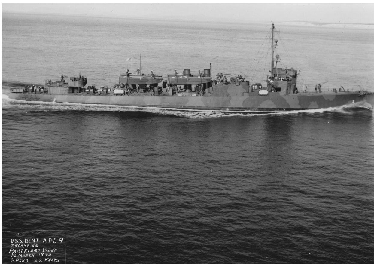
Figure 3 The USS Dent , March 1943, after her conversion to a fast troop transport ship, redesignated as APD-9. Note that two of her four stacks have been removed as have the twelve torpedo tubes, making space for four landing craft. Photo courtesy of Naval History and Heritage Command.
